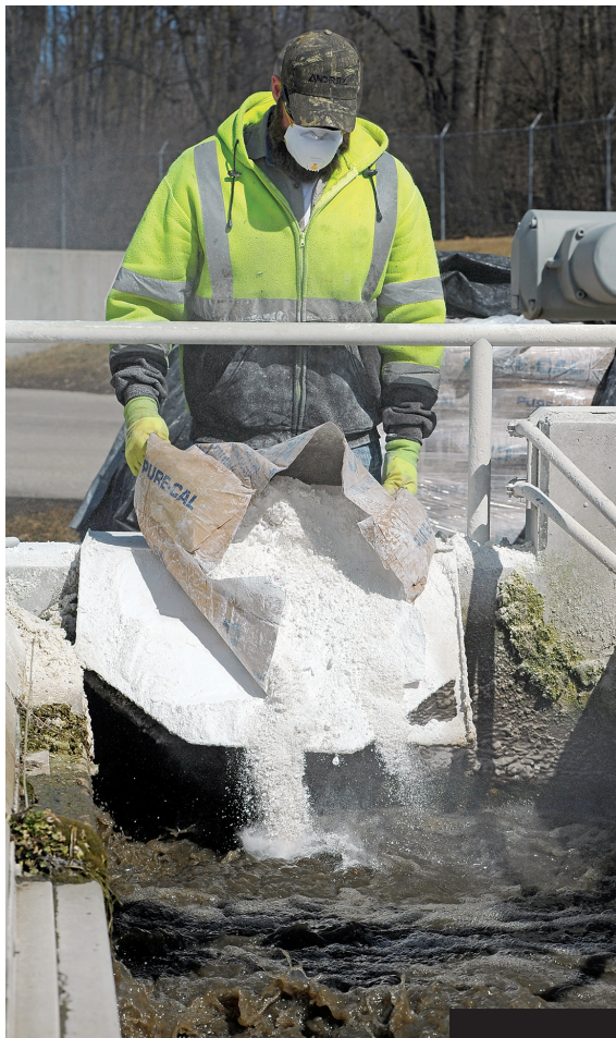
Joe Kell adds lime to the oxidation ditch twice a day as another technique for phosphorus reduction.
